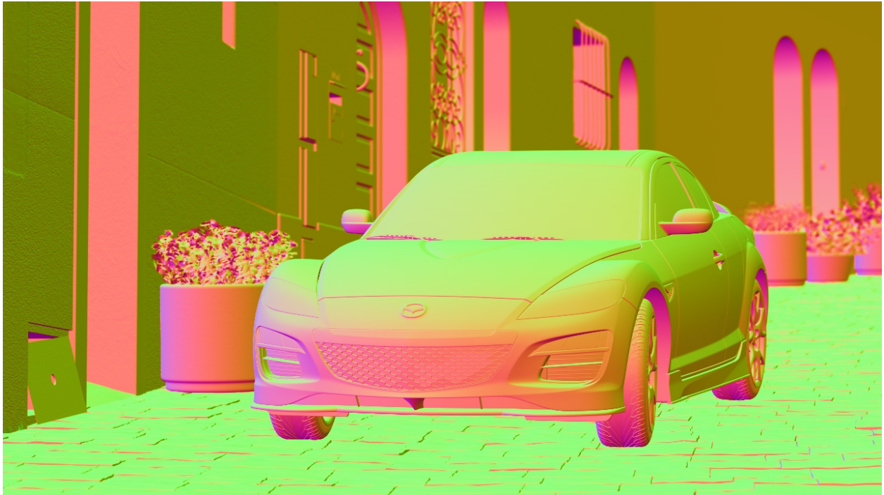
Fig. 7: Example normal image obtained using the first hit (the values are actually in [-1, 1] but were mapped to [0, 1] for illustration purposes).
